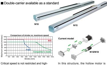
Critical speed is not restricted and highspeed transfer is possible. Stroke: 2500 mm Maximum speed: 1200 mm/sec. In this structure, the hollow motor is connected to the nut of the ball screw and the nut is rotated with the screw shaft secured to perform the movement.
